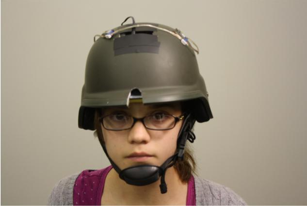
**Figure 1: An example near-axis retroreflective projector system in a military style helmet. Note the opening where the center axis of projection is located.**
