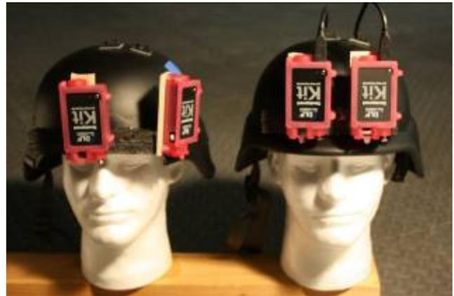
Figure 5: A projector configuration for a wider field of view (left) or for 3D stereoscopic imagery (right).
