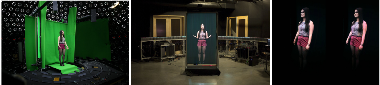
Figure 1: (left) Subject is recorded by an array of HD camcorders under controlled lighting. (Center) Subject shown on the automultiscopic projector array. The display can be seen by multiple viewers over a 135° field of view without the need for special glasses. (Right) Stereo photograph of the subject on the display, left-right reversed for cross-fused stereo viewing.
