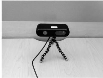
**Fig. 1.** PrimeSense Reference Design USB plug-and-play device
